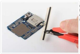
Cut the headers to length: Line the header strip up with the holes on the edge of the shield and cut 4 sections of header strip to fit.
