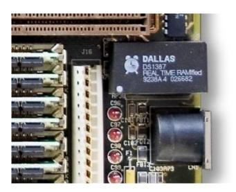
This image shows a computer motherboard with a Real Time Clock called the DS1387 (http://adafru.it/aX0). Theres a lithium battery in there which is why its so big.
