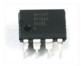
As long as it has a coin cell to run it, the DS1307 will merrily tick along for a long time, even when the Arduino loses power, or is reprogrammed.
