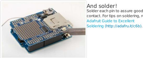
And solder! Solder each pin to assure good electrical contact. For tips on soldering, refer to the Adafruit Guide to Excellent
