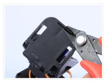
Cut a notch for the cable connectors We need to make room for the cable connectors on
