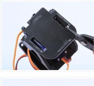
the back of the camera module. Two cuts, as shown in the photos will remove the top left side of the bracket.
