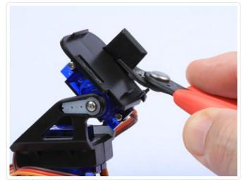
Trim the remaining tabs flush There are two smaller alignment tabs and a cable guide that must be trimmed flush also.
