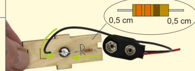
Solder the remaining red to the resistor and then carry out a visual check. After that, insert the
