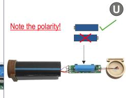
Slide the board into the tube
