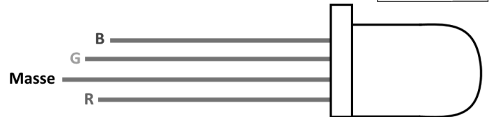
Connection pins of an RGB-LED
