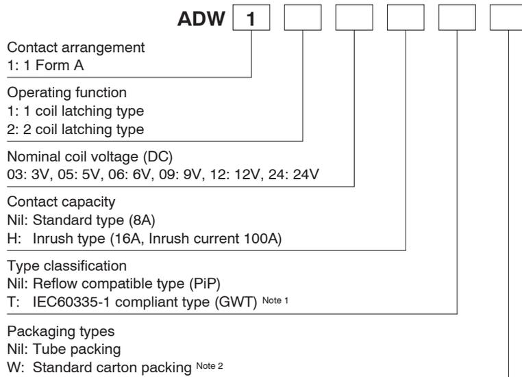
Notes: 1. T type is non-compliant for reflow soldering.
