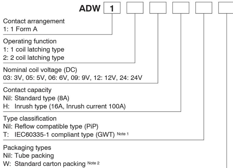
Notes: 1. T type is non-compliant for reflow soldering.
