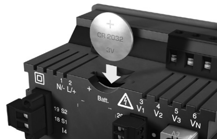
Fig. Battery insertion on the rear
