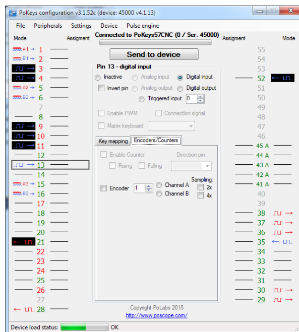
Figure 3: Encoder settings in PoKeys application
