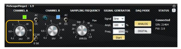
Since the analog generator outputs a voltage amplitude of no more than 2V, you can set the channel A knob to 2V. You will get graphical representation shown below.
