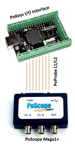
Logic analyzer measurements on PoKeys I/O controller
