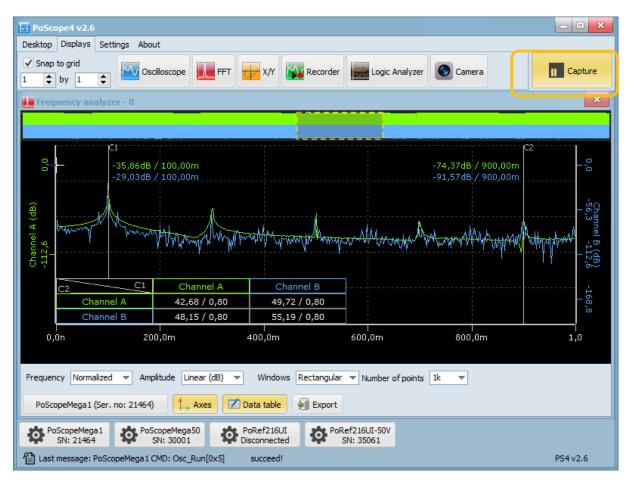
Frequency analyzer in Analyze mode with Overview window
