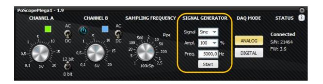
The waveforms on the oscilloscope display will change according to the shape of selected signal on the analog generator part of the Mega1 controls.
