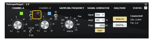
Channel B on/off button on Mega1 device controls
