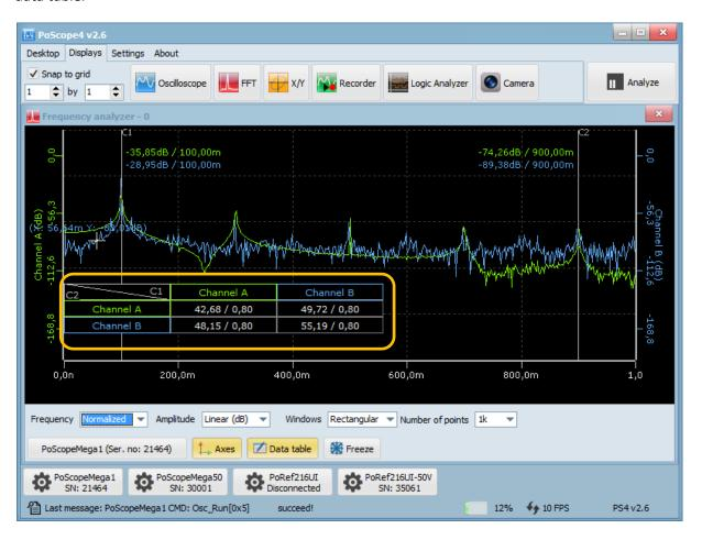
Frequency analyzer with data table open
