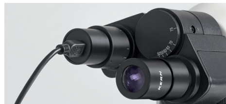
Eyepiece camera fixed into the tube
