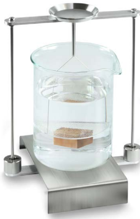
Fig. 4: Weighing in the auxiliary liquid
