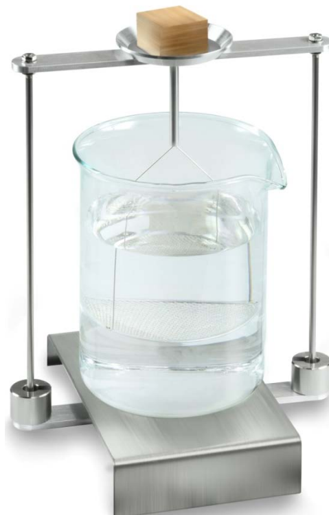
Fig. 3: Weighing in air
