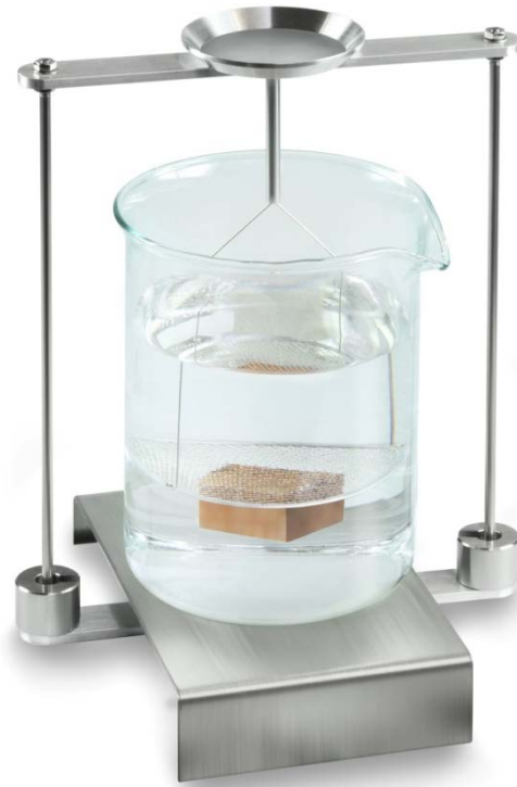
Fig. 4: Weighing in auxiliary liquid
