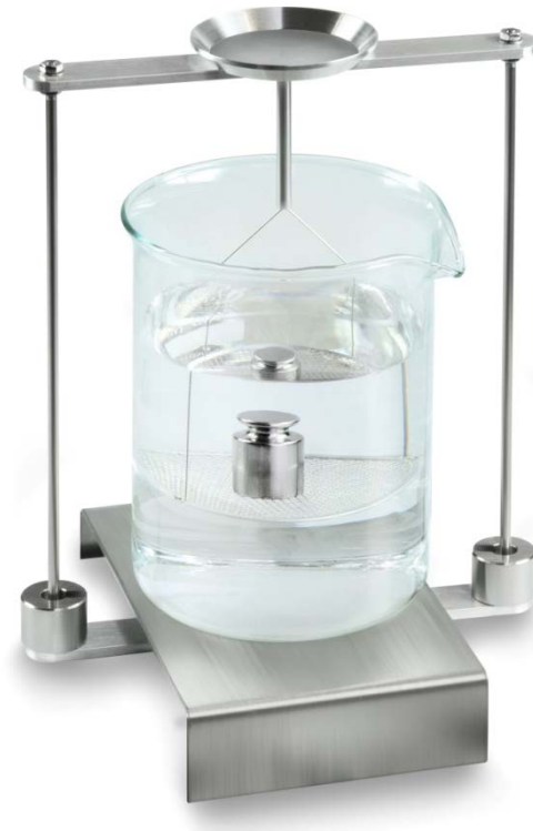
Fig.6: Weighing in test liquid
