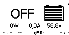
Fig. 7: Display after switching on the external battery fuse
