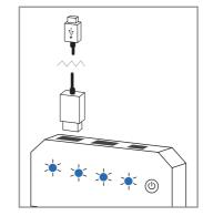
Attach any USB cable to either of the USB output sockets. Then connect the cable to the device that you wish to charge. Once your device is fully charged, the discovery will automatically turn off.
