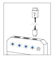
Connect the included cable to a 5V USB output socket (e.g. a laptop or wall plug with USB socket) and connect the micro USB end into the micro USB socket on the discovery. A full charge will take approx. 6 hours depending on the output of the USB port.
