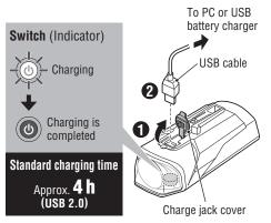
\* If the indicator flashes, there is a charging error. Remove the cable and try again.
