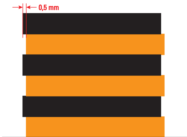
Front view of the 1st printout (offset X) Offset in X-direction in this example: 0.5 mm or 500 µm
