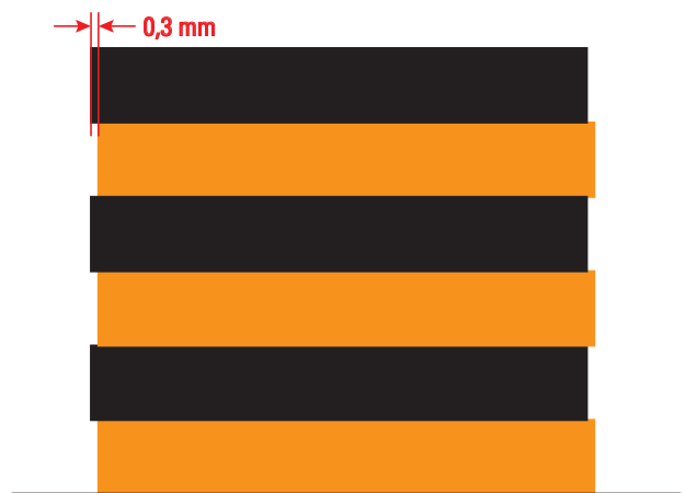
View from the right (offset Y) Offset in Y-direction in this example: 0.3 mm or 300 µm
