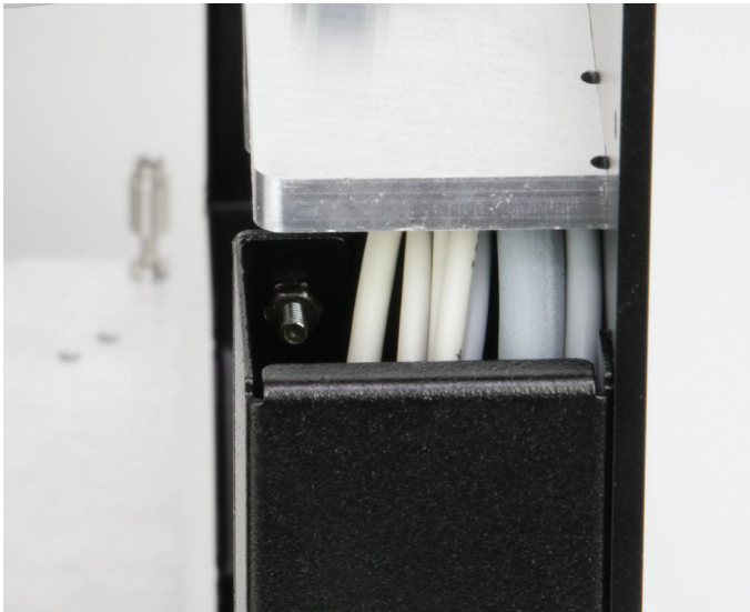
Fasten the upper cylinder head screw with a nut M4. It is best to use a small pointed pliers or tweezers first and an external hexagon socket wrench to tighten it.
