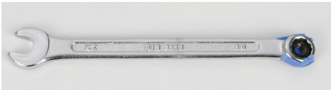
Fasten the cylinder head screw with the nut M4. If you do not have a suitable special tool, use a ring or fork wrench and tape one side with adhesive tape. You can then insert the nut from the other side and guide it to the screw. See figures below. Finally, reassemble the foot and holder.
