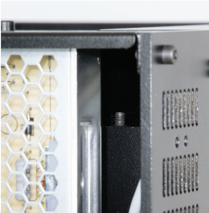
Fasten the cylinder head screw with the nut M4. If you do not have a suitable special tool, use a ring or fork wrench and tape one side with adhesive tape. You can then insert the nut from the other side and guide it to the screw. See figures below. Finally, reassemble the foot and holder.
