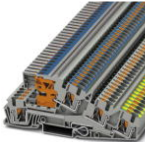
Installation ground terminal block, Push-in connection, Cross section: 0.2 mm 2 - 6 mm 2 , AWG: 24 - 10, Width: 6.2 mm, Color: gray, Mounting type: NS 35/7,5, NS 35/15
