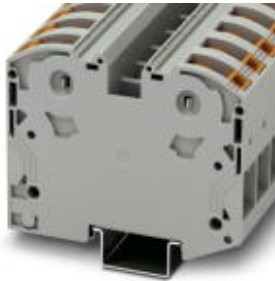
High-current terminal block, Connection method: Power-Turn connection, Number of connections: 2, Cross section: 2.5 mm 2 - 35 mm 2 , AWG: 12 - 2, Width: 16 mm, Color: gray, Mounting type: NS 35/15
