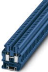
Mini feed-through terminal block, Connection method: Screw connection, Number of connections: 2, Cross section: 0.2 mm 2 - 4 mm 2 , AWG: 24 - 12, Width: 5.2 mm, Color: blue, Mounting type: NS 15
