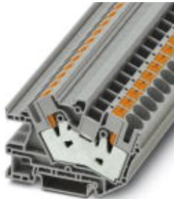
Installation terminal block, Push-in connection, Cross section: 0.5 mm 2 - 16 mm 2 , AWG: 24 - 4, Width: 10.2 mm, Color: gray, Mounting type: NS 35/7,5, NS 35/15
