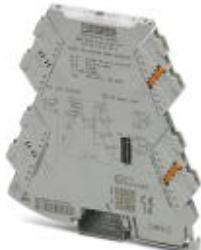
Output loop-powered 2-way isolator with plug-in connection technology for the electrical isolation of unipolar and bipolar analog signals. Input configurable via DIP switch. Push-in connection technology, standard configuration.
