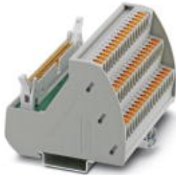
VARIOFACE module, with push-in connection and flat-ribbon cable connector, for mounting on NS 35 DIN rails, with pin strip plus short and long locking latches for socket strips, 26-pos.
