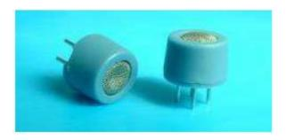
This item operates on the catalytic combustion principle, and its two arms of electric bridge consists of a test element and a compensate element. The resistance of the test element rises when meeting the combustible gas, in the same time, the output voltage of the bridge changed, the voltage variable is rise in direct proportion as the gas concentration, the compensate element as a reference, and compensate of temperature and humidity.
