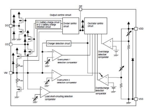
Remark All the diodes shown in the figure are parasitic diodes.
