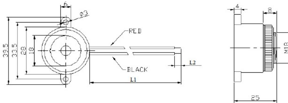
Lead wire: UL1007AWG26    L1: 150 ± 10mm    L2: 5.0 ± 2 mm
