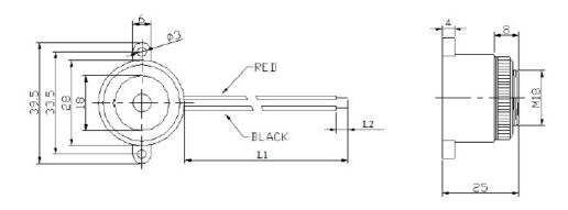
Lead wire: UL1007AWG26 L1:  $150 \pm 10$ mm L2:  $5.0 \pm 2$  mm
