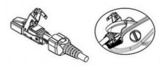
6. Close plug cover, make sure the drain wire is in proper contact with grounding clip. Pull back strain relief boot to cover the plug, fasten nylon cable tie to secure grounding contact.
