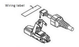
5. Place the wiring cap onto plug, use plier to clamp wiring cap until it is completely snap-in to effect the connection
