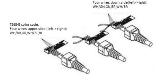
Remove the wiring label before place wiring cap on plug
