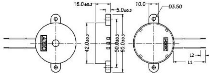
Lead Wire: UL 1007 AWG26 L1:125±5mm L2:5±2mm
