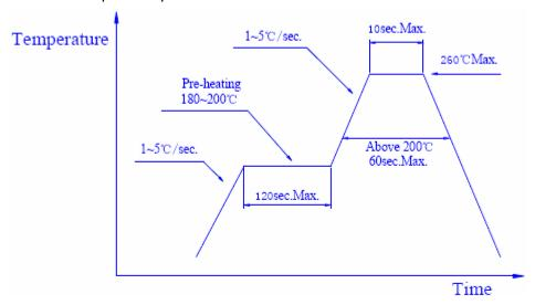
Reflow soldering should not be done more than two times When soldering, do not put stress on the LEDs during heating After soldering, do not warp the circuit board
