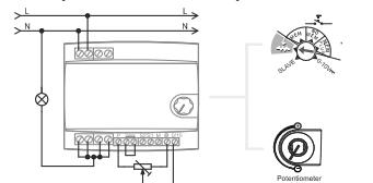
**B) Operation with int. potentiometer**
