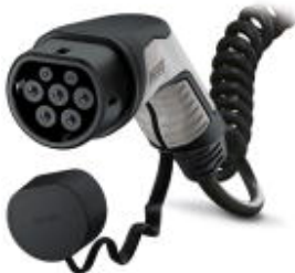
AC charging cable with Vehicle Connector, open cable end, with protective cap, Type 2, IEC 62196-2, 20 A / 480 V (AC), Design line C-Line, Cable: 4 m, black, spiraled, Mating face: black, Handle area: gray
