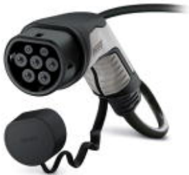
AC charging cable with Vehicle Connector, open cable end, with protective cap, Type 2, IEC 62196-2, 20 A / 250 V (AC), Design line C-Line, Cable: 5 m, black, straight, Special version with individual ferrules, Mating face: black, Handle area: gray
