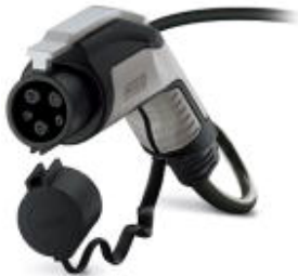
AC charging cable with Vehicle Connector, open cable end, with locking option for U-lock, with protective cap, Type 1, IEC 62196-2, SAE J1772, 20 A / 250 V (AC), Design line C-Line, Cable: 5 m, black, straight, Mating face: black, Handle area: gray
