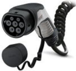
AC charging cable with Vehicle Connector, open cable end, with protective cap, Type 2, IEC 62196-2, 20 A / 250 V (AC), Design line C-Line, Cable: 4 m, black, spiraled, Mating face: black, Handle area: gray
