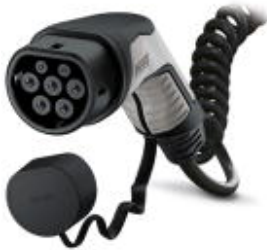
AC charging cable with Vehicle Connector, open cable end, with protective cap, Type 2, IEC 62196-2, 32 A / 250 V (AC), Design line C-Line, Cable: 4 m, black, spiraled, Mating face: black, Handle area: gray
