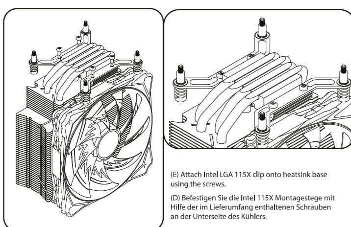
(E) Attach Intel LGA 115X clip onto heatsink base using the screws.
