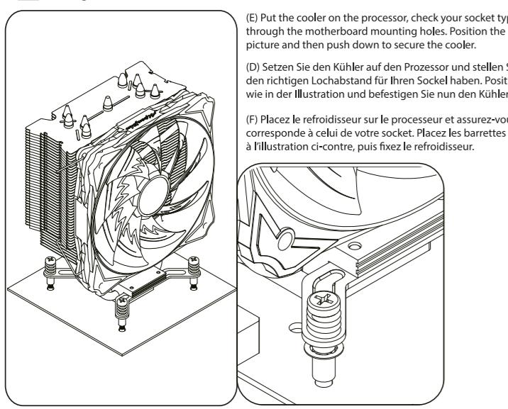
(E) Put the cooler on the processor, check your socket type and ensure all screws through the motherboard mounting holes. Position the clip as shown in the picture and then push down to secure the cooler.
