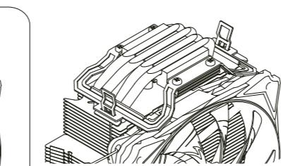
(E) Attach the AMD metal clips onto heatsink base using the screws.
