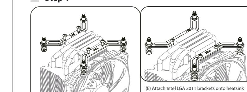
(E) Attach Intel LGA 2011 brackets onto heatsink base using the screws.
