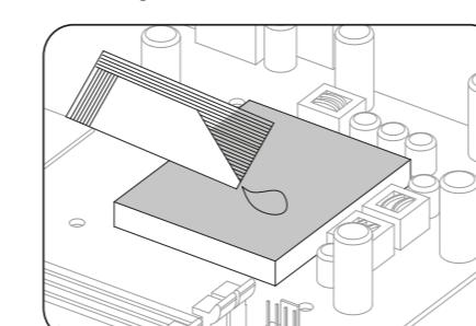
(E) Evenly apply a thin layer of thermal grease onto the processor.
