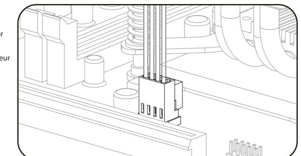
(E) Finish the installation by connecting the fan cable to the motherboard.
