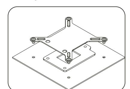
(E) Will provide the backplate installed to the motherboard on the back of the upper part, placed correctly on the motherboard back.
