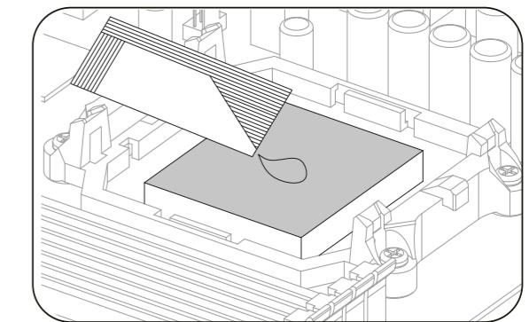
(E) Evenly apply a thin layer of thermal grease onto the processor.
