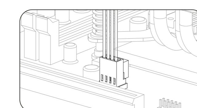
(E) Finish the installation by connecting the fan cable to the motherboard.
