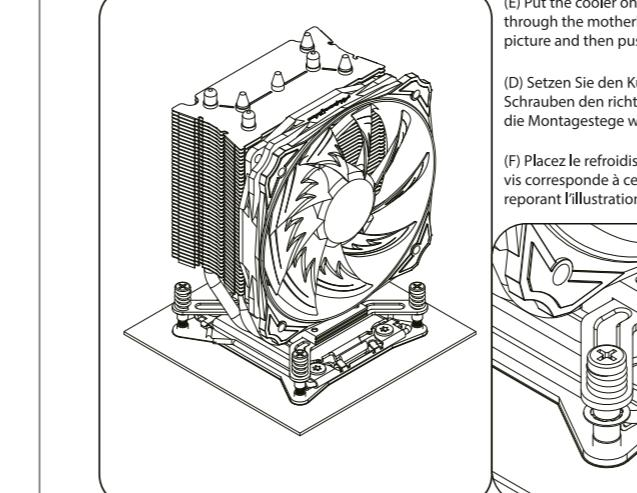
(E) Put the cooler on the processor, check your socket type and ensure all screws through the motherboard mounting holes. Position the clip as shown in the picture and then push down to secure the cooler.
