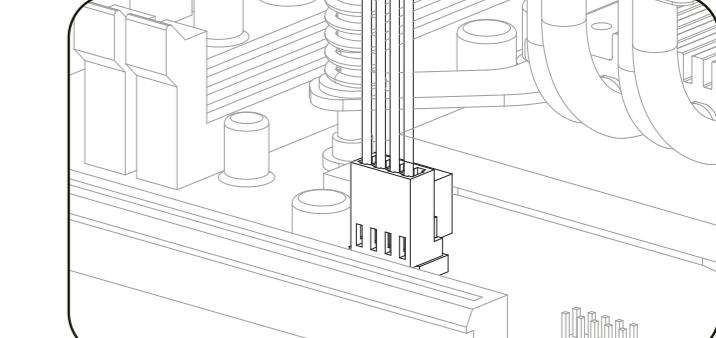
(E) Finish the installation by connecting the fan cable to the motherboard.
