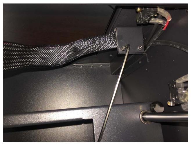
•8. Lay the RF100 3D printerand then lossen 4 bottom screws with rubber feet by allen key 3.0mm.
