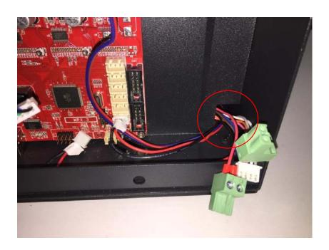
•21. Pull the X-axis motor cable and limit switch cable out of the nylon sleeve. . (SR20170621 pull out te cables out from ribbon cable carefully. One side is still connected to motor)
