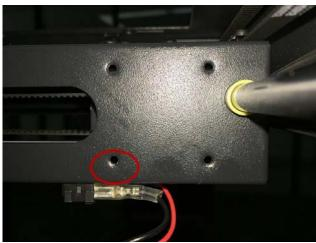
•30. Use cable holder 01 and M3\*8 screw and washer to fix on the hole. (90 degree angle)
