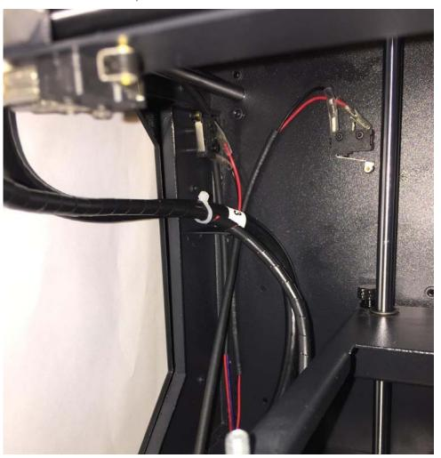
•37. Use cable holder 02 and M3\*8 screw and washer to fix.
