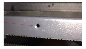
•28. Then use the cable holder 01 and M3\*6 screw and washer to fix on the middle of X-axis frame hole.( Lisa: fix the part of cable 1 with the cable holder to the middle of the x –axis. For this place the cable between the cable
