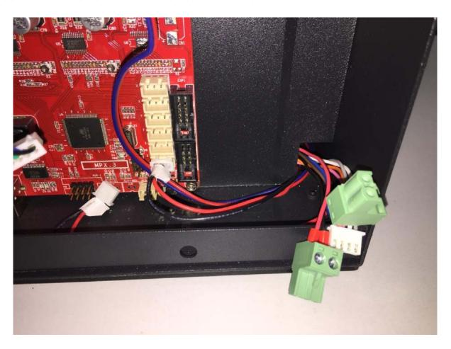
•34. Use cable ties and fix both cables as shown in the picture.and cut off the remaining part.
