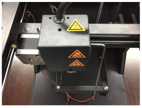
•25.Place the L shape metal stand (Lisa: spare part of the cable set) to extruder cover and tighten the two M3\*6 screws (Lisa: = part of the cable set) by allen key 2.5mm.
