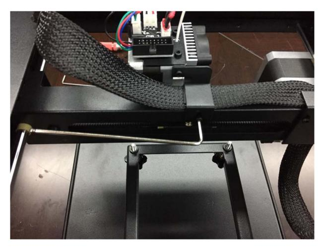
•5.Remove the metal bracket 02 by allen key 2.5mm
