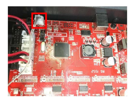
•14.Remove extruder & X-axis motor power cable from the terminal.
