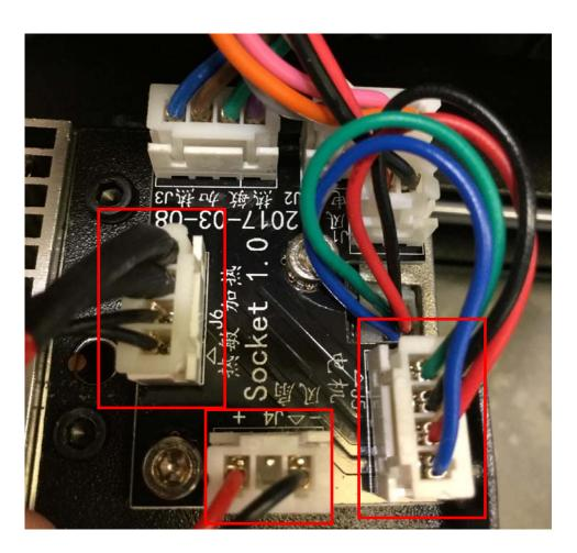
•22 unscrew (screw size needed) and remove the old exturder PCB from Extruder unit. Replace this with the new round cable PCB Fix the new pcb with 2 screws by allen key 2.5mm. Screw photos needed
