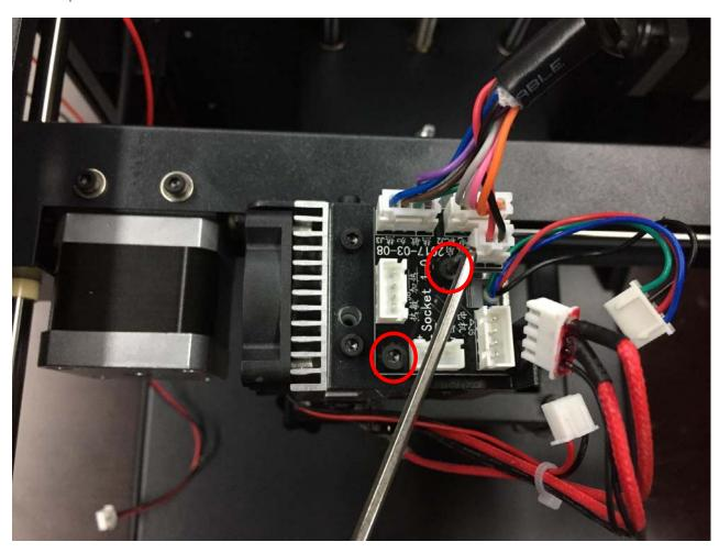
•23. Plug the connector removed in (previous 2 steps) to the new PCB. Correct connection as shown below.
