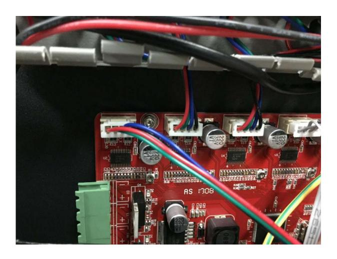
•41. Reinstall the thermistors cable and limit switch cable as shown in the picture.
