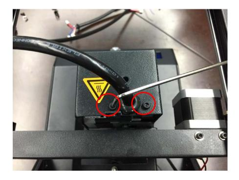
•26. Fix cable holder 01 with M3\*8 screw and nut on cover stand by allen key 2.5mm.
