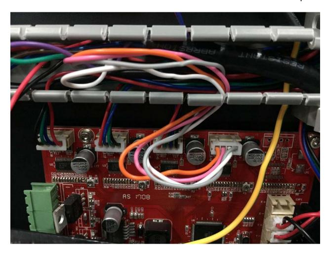
•40. Reinstall the X axis motor able to terminal as shown in the picture
