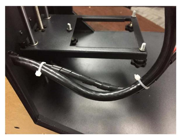
•36. Place cable that sticker 03 will fit to the reference position as shown in the picture (left frame/ left side of build bed) .
