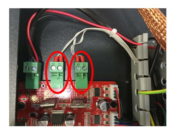
•13.Remove the thermistors cable from the terminal.
