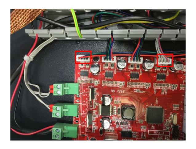
•17. plug off X-axis limit switch cable from the terminal.
