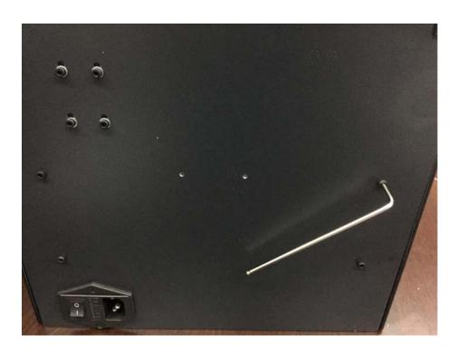
•38. Through all round cable terminals to the hole (in the corner) until we can see all of them at the bottom. (carefully, one by one terminator)
