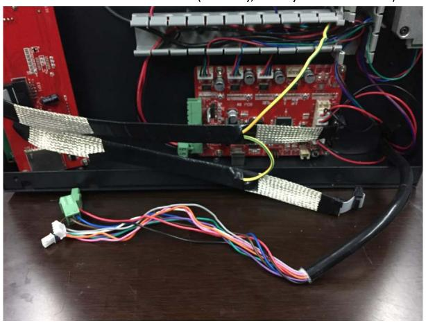
•39. Reinstall the extruder motor cable to terminal as shown in the picture.
