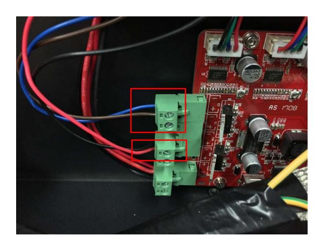
•44. Reinstall the cable with metal protector as shown in the picture. (take care that the cable should not be twisted. They should be plug in parallel)
