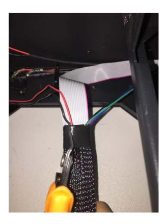
20.Pull the ribbon cable and cables out from the bottom (back) of printer through the opening carefully, so other cables are not damaged. ATTENTION the terminal only fits through the hole one by one
