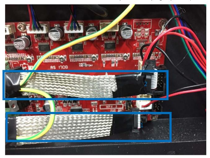
•45. Put the cable back into the cable slot to make them in order.
