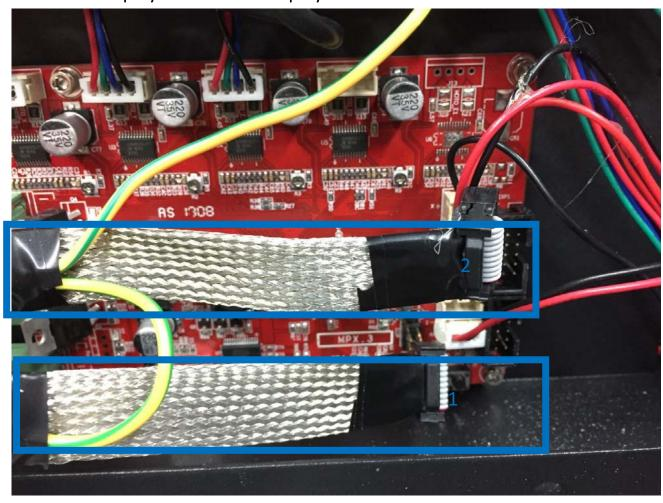
•12. plug off the 2x heating port and fan power cable from the terminal.
