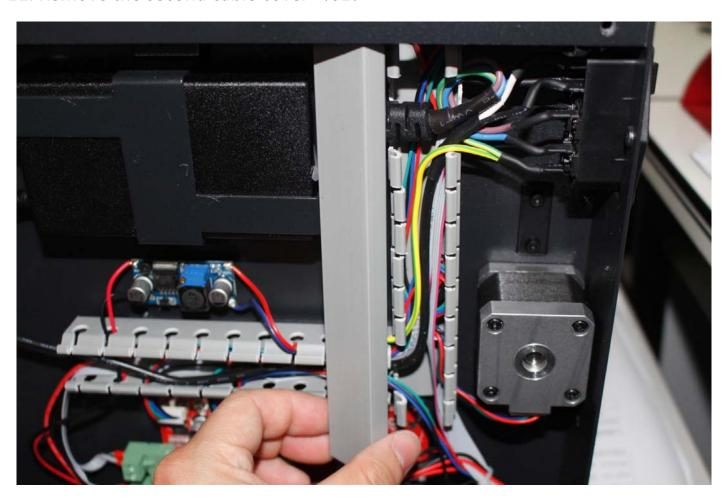
•15. Remove display PCB 01 and display PCB 02 cable .
