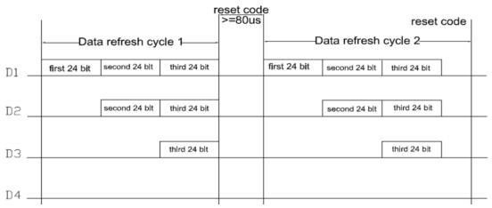
Note: the D1 sends data for MCU, D2, D3, D4 for data forwarding automatic shaping cascade circuit.
