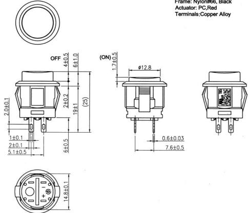
Tolerances Unless Otherwise Specified ±0.3 Unit: mm
