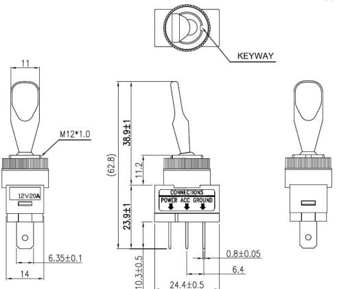
1 . Tolerances ±0.3 Unless Otherwise Specified Unit: mm
