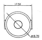
Frame: Nylon66 94V-0 BK Actuator: Nylon66 94V-0 BK Terminal: Silver Plated Brass Operation Force:100±25gf
