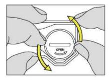
■ Put CR2032 battery into battery house, the positive side of battery (+) should face out.
