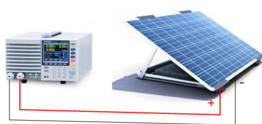
Connections Between PEL-3041 and Solar Panel
