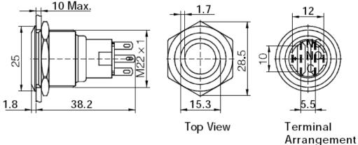
10 MAX: means the panel thickness, the max thickness for the panel no more than 10mm.
