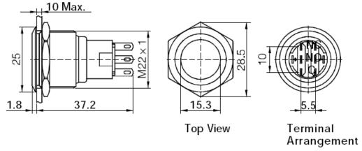
10 MAX: means the panel thickness, the max thickness for the panel no more than 10mm.
