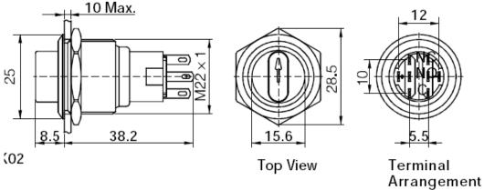
10 MAX: means the panel thickness, the max thickness for the panel no more than 10mm.
