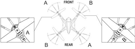
\* Please unscrew the screw for the blade before replace the blade.
