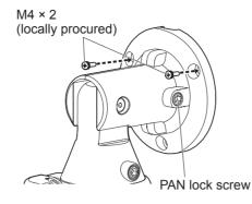
2 Use the 2 upper M4 screws (locally procured) to secure the camera. And then loosen the PAN lock screw about 1 turn.
