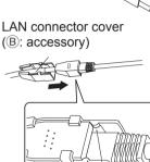
The hook engages with the connector terminal
