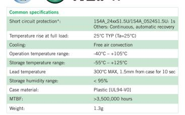
$<sup>^{*}</sup>$  Supply voltage must be discontinued at the end of short circuit duration for models 1S4A\_24xxS1.5U and 1S4A\_0524S1.5U.
